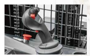
The multi-function control handle's unique shape and angled design helps to minimize hand movement and muscle fatigue.
