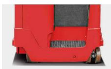
The operator is able to get on and off the truck more comfortably thanks to the low step-on height of the reach truck's operator compartment.
