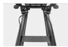
The lifting system is optimized for the operator to have an excellent line of sight through the mast.
